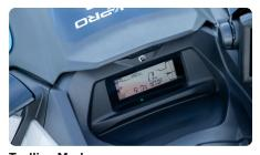
**Trolling Mode** Enables precise control of speed. Choose one of several presets and adjust as needed.
